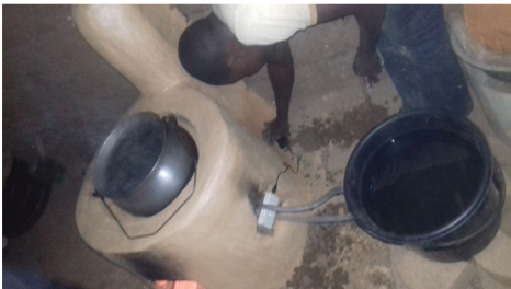
Wanrou cookstove in combination with a Electric Thermo Generator charging mobile phone and LED lamps (in partership with Trinity College Dublin)
