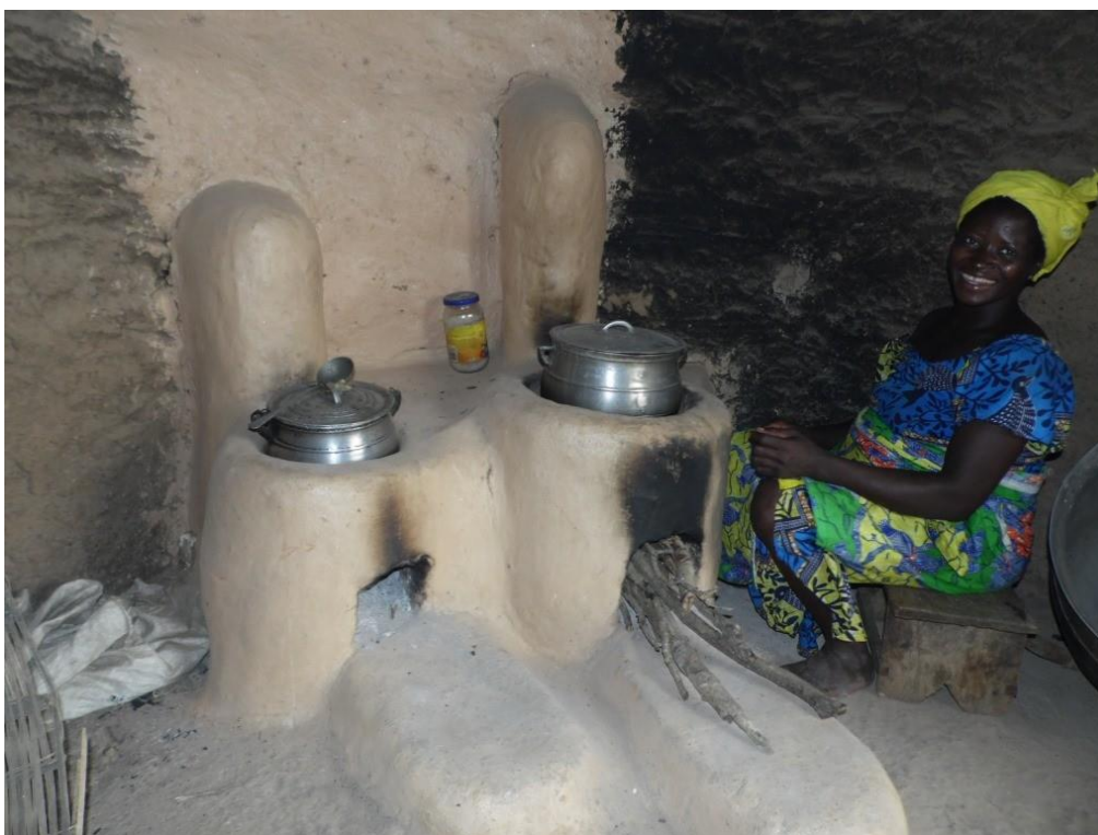
Wanrou efficient cookstove with chimney and separated combustion chamber
